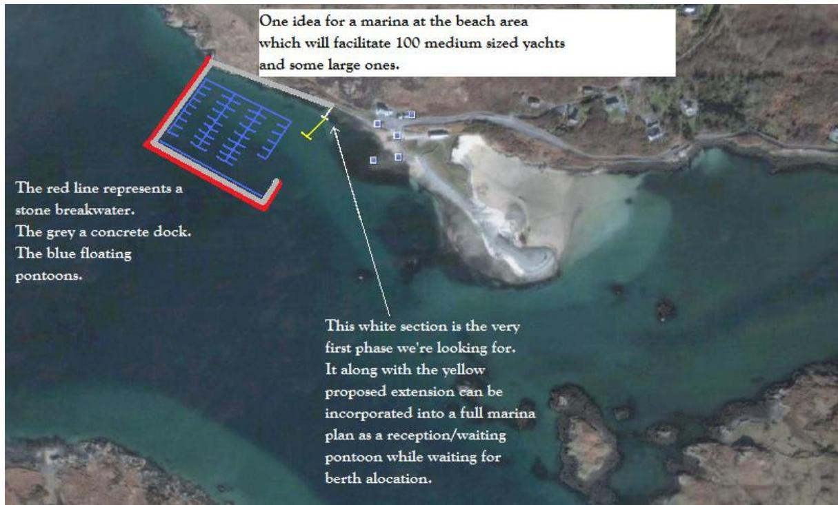
This would involve building a proper breakwater (drawn here in red), from stone or other recommended materials, to protect the marina inside.
